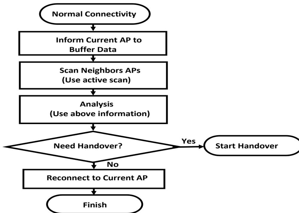
Figure 1: Proactive Scanning Phase Flowchart
